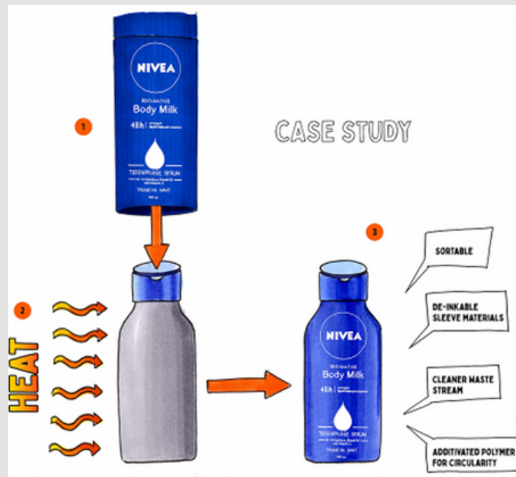
Image: Design4Circularity initiative has created a colourless polyolefin bottle made from 100% post-consumer recycled material. (Source: PlasticsToday.com)
